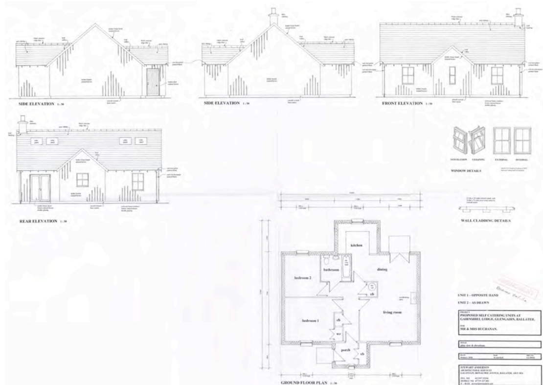
Fig. 4. Chalet Unit Elevations and Floor plan
